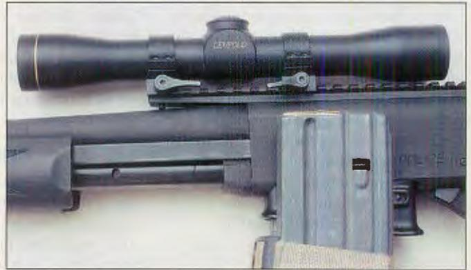
*(above) Leupold's Scout Scope found a perfect place on the Krebs M1913 Extended Rail. (below) Here Leupold's new MR/T 3-9X Scope is seen mounted on the 7615P using A.R.M.S. QD ThrowLever Rings. The MR/T has an illuminated reticle and is identical to the TX-30A2 now in use with SF in Afghanistan and Iraq.*
